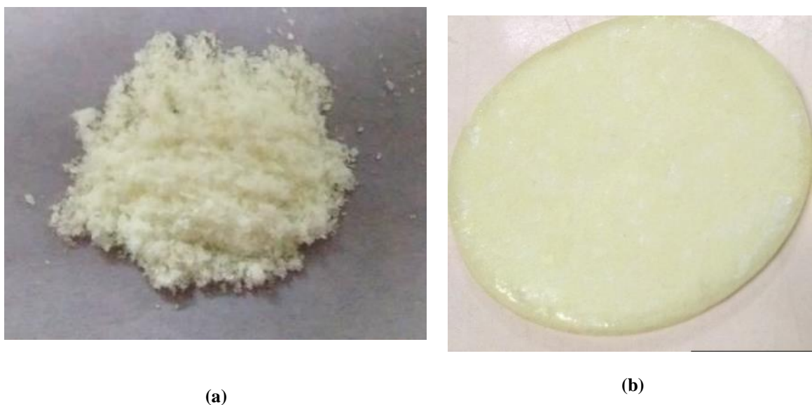
Figure 3. Dry powder Ca-Alginate beads (a) and Patch using dry powder Ca-Alginate beads as a drug reservoir.
